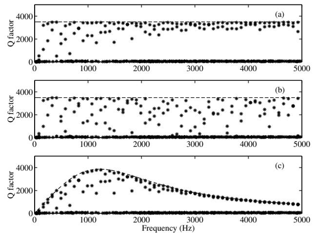
Figure 6. Computed  $Q$ -factors from three different synthesis methods: (a) the first-order modal method, assuming constant string damping; (b) the undamped modal method plus Rayleigh’s principle, assuming constant string damping; (c) the first-order modal method using frequency-dependent string damping as determined from measurements [1]. In each case the dashed line shows the string damping as a function of frequency. The low- $Q$  modes near the horizontal axis are “body modes”.
