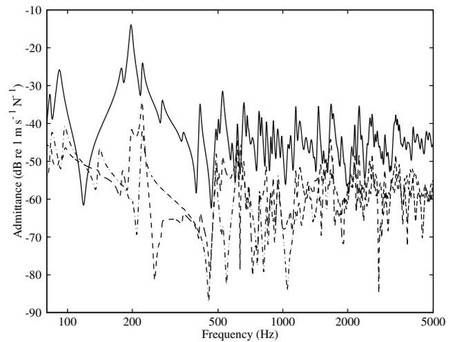
Figure 3. Calibrated admittances  $Y_{11}$  (solid line),  $Y_{12}$  (dashed line) and  $Y_{22}$  (dash-dot line) determined from a test guitar by measurement followed by modal fitting, as described in the text and more fully in [1].
